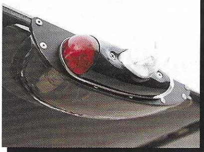
Top of the line strobes from Whelen are 3 lights in one: strobe, navigation and position.
