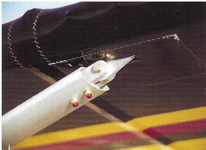
Streamline struts and CNC machined fittings are standard.
